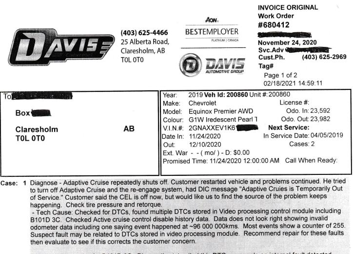
Followed diagnostics for B101D 3C. Diagnostic states that this DTC represents an internal fault detected within the module. - Tech Comments: Recommend replace Video Processing Control Module.
