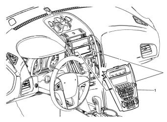
4. Remove the radio control assembly (1). Refer to Radio Control Assembly Replacement in SI.
