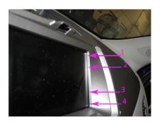
1. Visually inspect the complete area around the rectangular radio touch screen for insufficient clearance as shown (1), (2). Compare to the area with sufficient clearance (3), (4) in order to make a determination of where to apply the loop tape.
