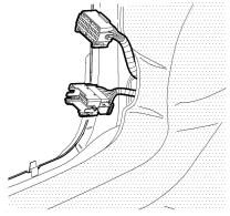
3. Disconnect the instrument panel/body inline connector (black 40-pin electrical connector).
