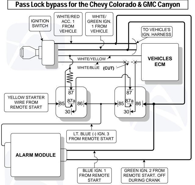
The above diagram shows you how to bypass the PASS LOCK system on the Chevy Colorado & GMC Canyon. This system is different from previous PASS LOCK systems. Below is the procedure for bypassing the PASS LOCK when installing a remote start.
