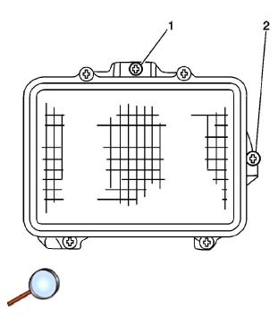
Correct the horizontal aiming and the vertical aiming of each headlamp by adjusting the screws. The screws move the mounting bracket against the tension of the coil spring. The screws are in the headlamp bezel area on the models with the sealed beam headlamp.
