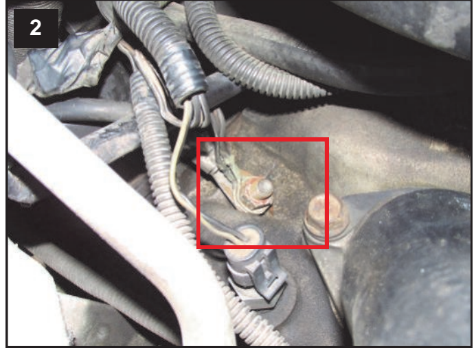
Unknown Engine Ground. May be G104. Top Front of Engine Block just Right of Thermostat Housing.
