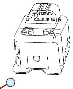
2. Install the inside air temperature sensor to the headliner and sensor grille.
