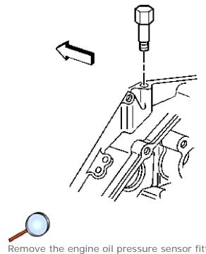
4. Remove the engine oil pressure sensor fitting, if necessary.
