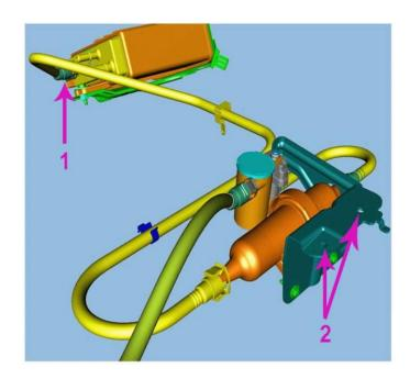
9. 2008-2009 Hybrid Models: Disconnect the CVS valve assembly quick connect fitting (1) from the EVAP canister.
