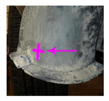
14. Drill a 7 mm (0.27 in) hole in the fuel tank filler pipe housing approximately 15 mm (0.59 in) back from the base of the flange and 15 mm (0.59 in) rearward of the forward housing attachment clip as shown.
