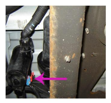
6. 2008-2009 Hybrid Models: Disconnect the vehicle chassis wiring harness electrical connector from the CVS valve.
