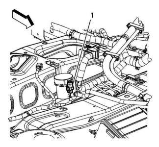
5. Disconnect the vehicle chassis wiring harness electrical connector (1) from the CVS valve.
