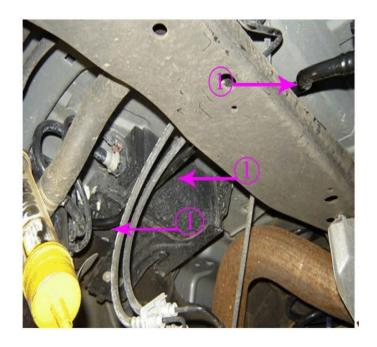
The revised CVS valve assembly EVAP canister pipe (1) MUST BE ROUTED ABOVE the cross-car brace, just forward of the CVS valve and BELOW the EVAP canister, as shown, rather than above the EVAP canister, as the original pipe was routed.
