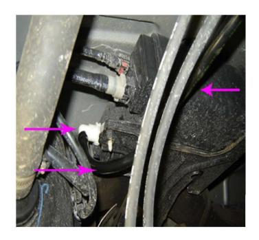
21. Connect the CVS valve assembly canister pipe quick connect fitting to the EVAP canister.
