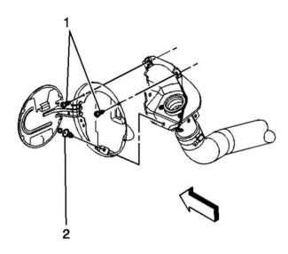
26. Install the <u>fuel tank</u> filler housing to body TORX(R) screws (1) and retainer (2).
