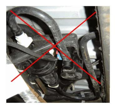
Shown is the original 2008-2009 EVAP canister vent solenoid (CVS) assembly used on hybrid fullsize utility vehicles. This assembly will be removed and discarded.
