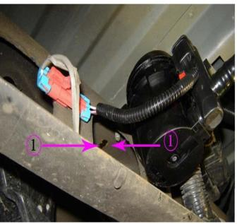
16. Position the CVS valve bracket anti-rotation tab (1), (shown on the workbench and installed in the vehicle), and fully seat it to the spare tire cross-car support.
