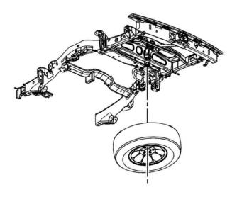
4. Remove the spare tire and wheel assembly.
