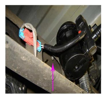
17. Install the bolt for the CVS valve assembly bracket, into the spare tire cross-car support as shown.
