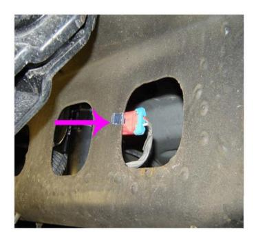
19. Secure the clip on the CVS valve jumper harness electrical connector to the spare tire crosscar support as shown.
